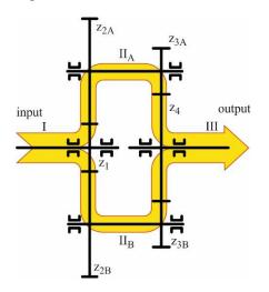
Fig. 1. A diagram of dual-path gear transmission (developed view), I – input shaft, II<sub>A</sub>, II<sub>B</sub> – intermediary shafts, III – output shaft,  $z_1$  – teeth number of pinion,  $z_{2A}$ ,  $z_{2B}$  – teeth number of wheels on shafts II,  $z_{3A}$ ,  $z_{3B}$  – teeth number of pinions on shafts II,  $z_4$  – teeth number of wheel on output shaft
