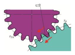
Fig. 4. The area of mashing B from Figure 2;  $\varepsilon$  – circumferential backlash
