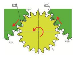
Fig. 3. The area of mashing A from Figure 2;  $\varepsilon$  – circumferential backlash
