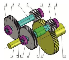
Fig. 7. A 3D view of the gear transmission; 1 – input shaft, 2 – pinion  $z_1$ , 3 – gear  $z_{2A}$ , 4 – gear  $z_{2B}$ , 5 – shaft II<sub>A</sub>, 6 – shaft II<sub>B</sub>, 7 – pinion  $z_{3A}$ , 8 – pinion  $z_{3B}$ , 9– gear  $z_4$ , 10 – shaft III, 11 – bearings
