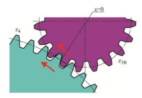
Fig. 5. The area of mashing C from Figure 2;  $\varepsilon$  – circumferential backlash
